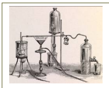
Apparatus for the detection of chloroform by the Ragsky process Arthur P. Luff, Text-book of forensic medicine and toxicology, 1895
